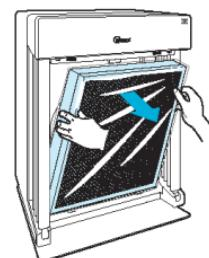
**③ Remove filters from protective plastic wrap.**
