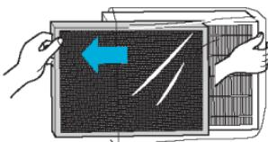
**④ Install the filters until they fit securely in place.**
